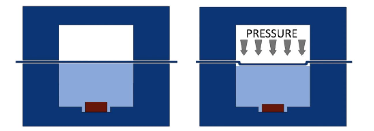
Hydrostatic compression of the specimen (red) is achieved by filling the culture well to the top with media. Pressurizing the top chamber results in the flexible membrane (black line) deflecting downwards to press against the surface of the liquid.
