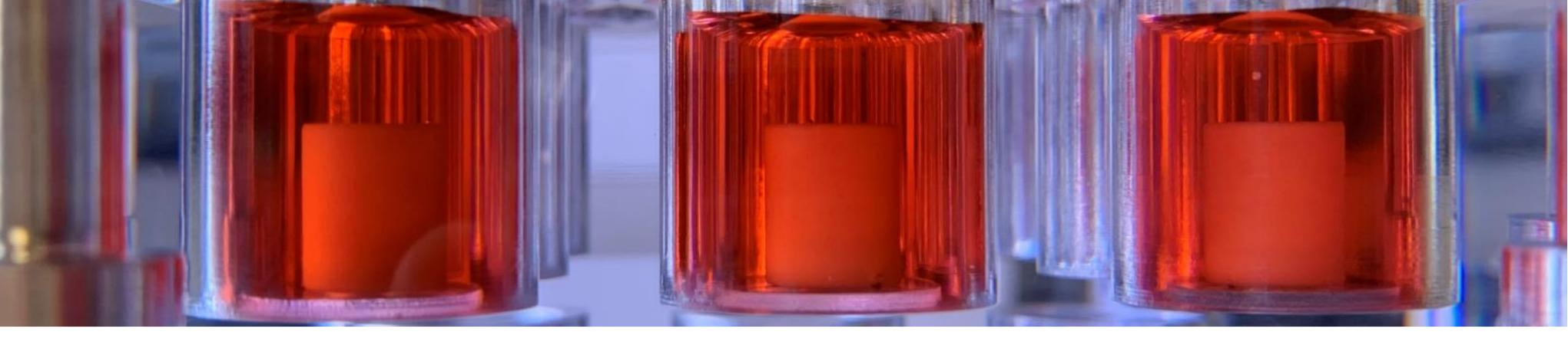
The MechanoCulture TR can be programmed to run constant velocity or sinusoidal compression patterns. Magnitudes, frequencies, rest periods, and cycle counts can all be specified in the software application and programmed to the device.
